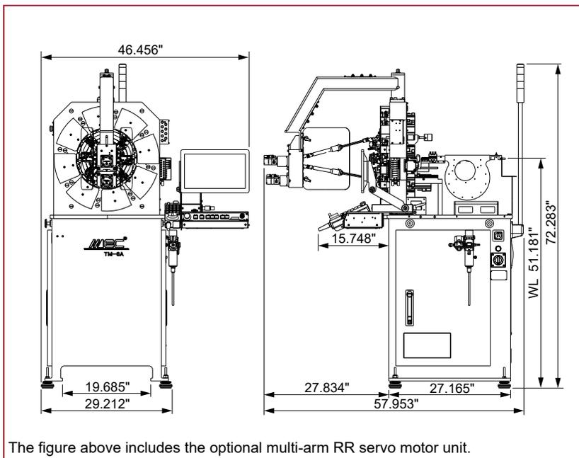
The figure above includes the optional multi-arm RR servo motor unit.
