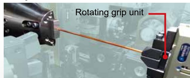
The rotating grip unit can be also used for long length forming.
